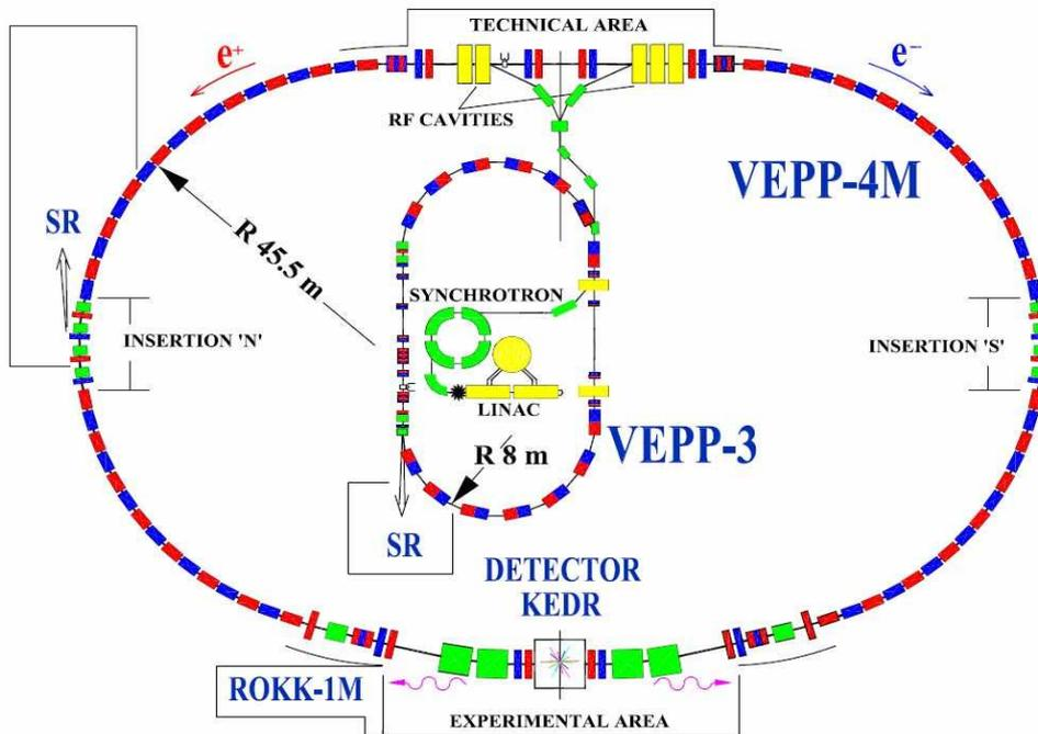
Figure 1: Layout of the VEPP-4 facility.
