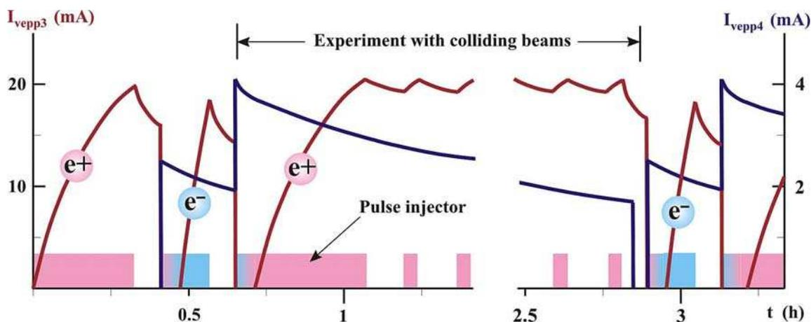
Figure 4: Diagram of the VEPP-4 operations in the mode of the experiment with colliding beams.
