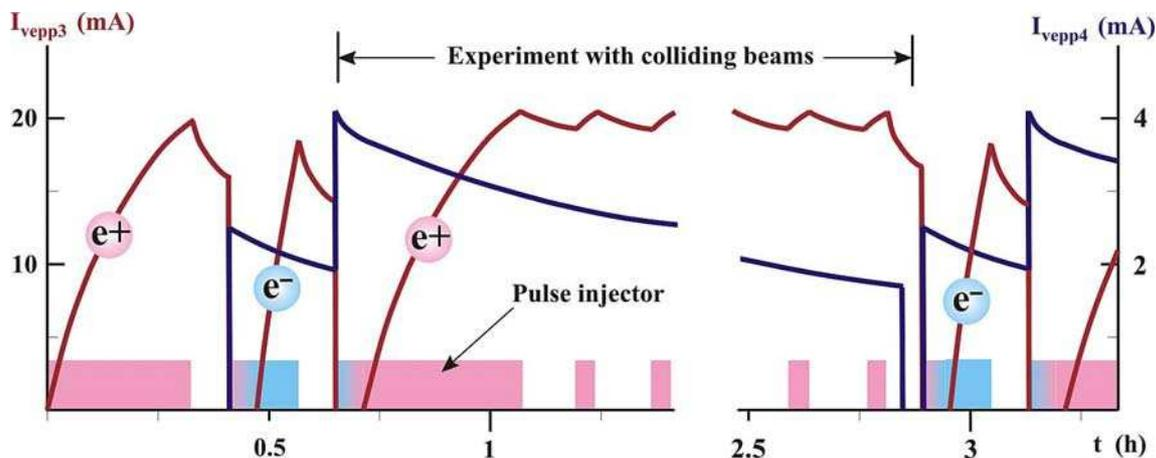
Figure 4: Diagram of the VEPP-4 operations in the mode of the experiment with colliding beams.
