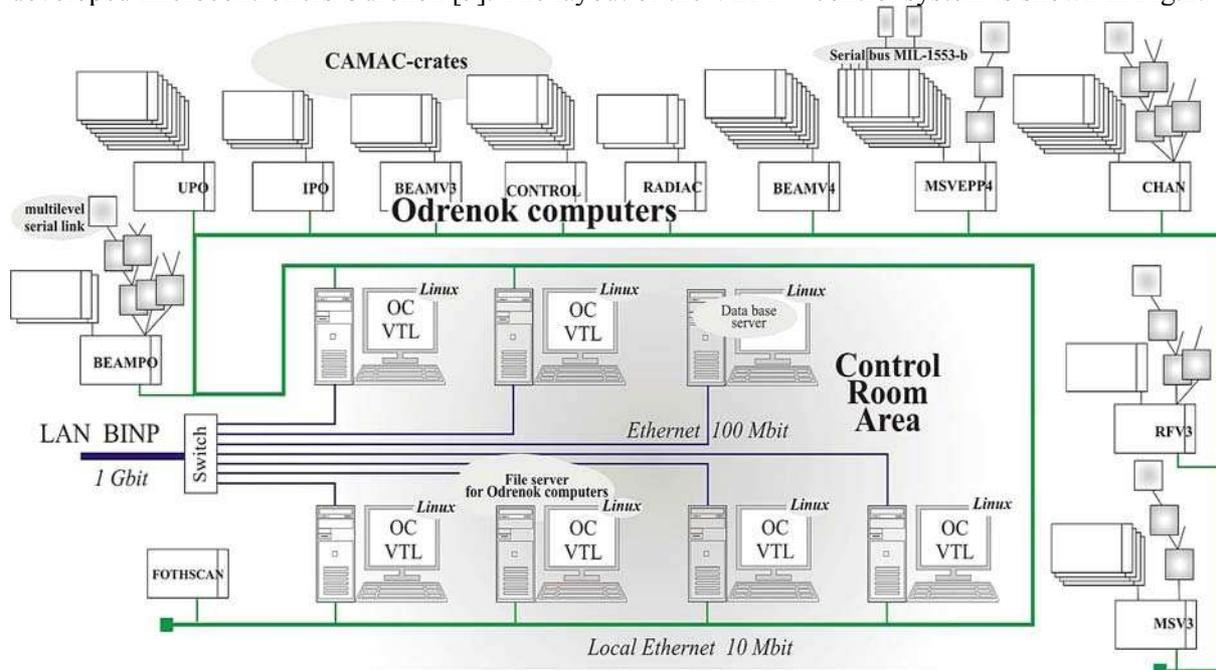
Figure 2: The layout of the VEPP-4 control system.
