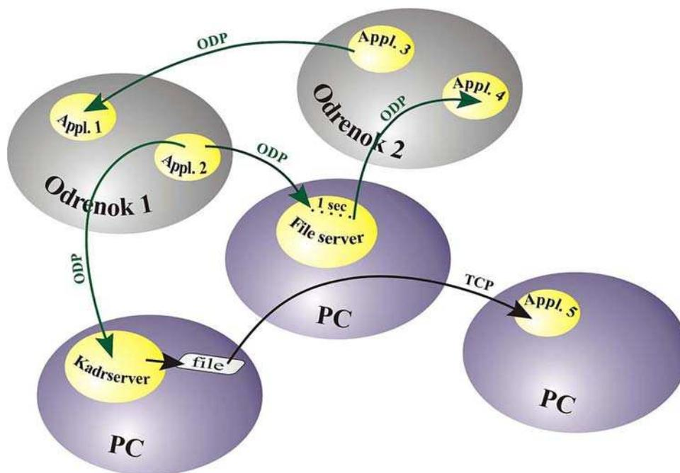
Figure 3: The methods of data exchange in the VEPP-4 control system.
