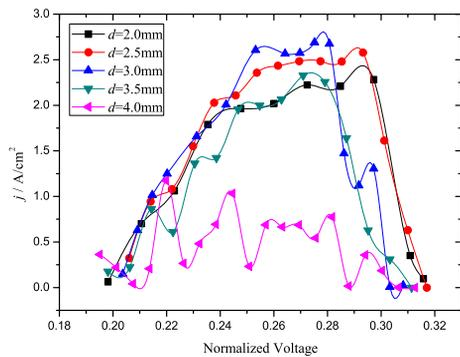
Figure 3: Maximal current destiny with different cathode-grid distance.
