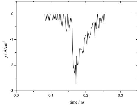
Figure 2: Output current destiny of a RF cycle.
