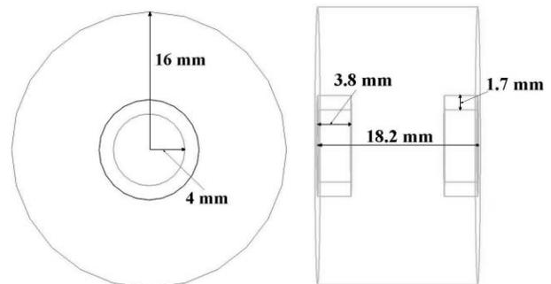
Figure 5: Optimized geometry of the 6 GHz cavity.
