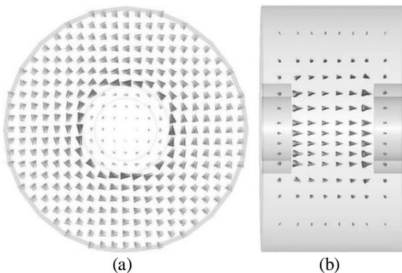
Figure 7: Field distributions of the 6-GHz prebuncher
