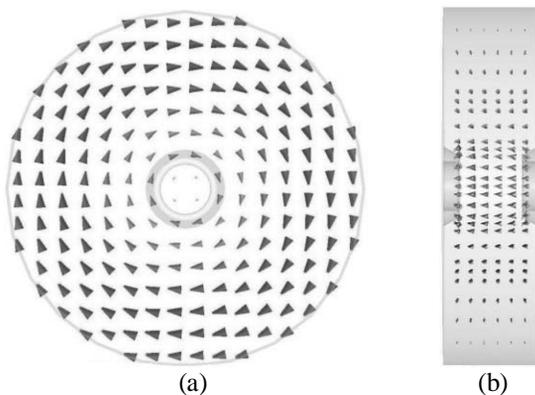
Figure 6: Field distributions of the 3-GHz prebuncher
