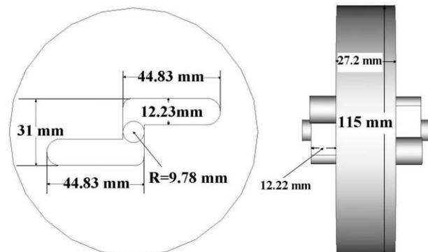
Figure 1: Optimum geometry of the chopping cavity.
