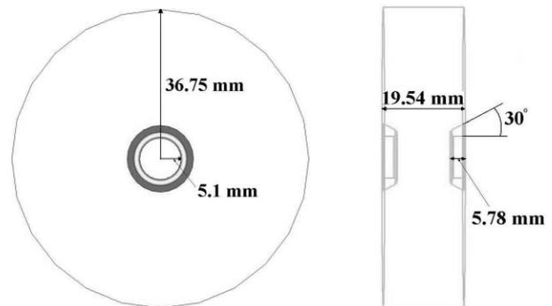
Figure 4: Optimized geometry of the 3 GHz cavity.
