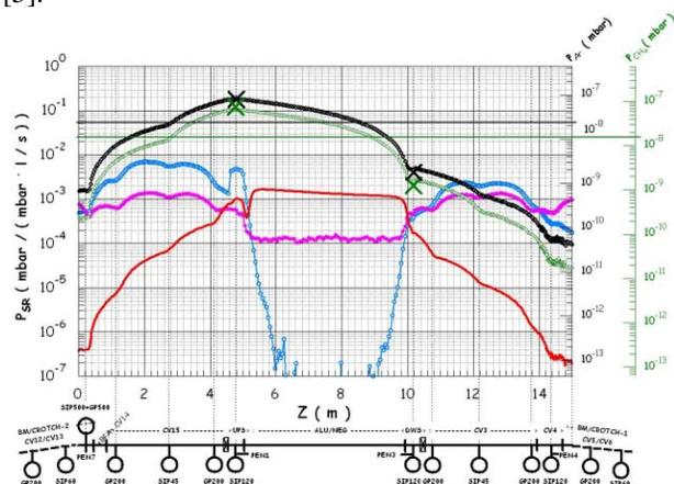
Figure 1: MC calculation of the pressure profiles for Ar (black), CH<sub>4</sub> (green), scales on the right. Thermal (magenta), and SR-induced gas loads (red and blue, for UPS/ID chambers only, and all other absorbers, respectively), scale on the left.
