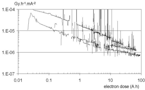
Figure 3: Gas-bremsstrahlung measurements during initial vacuum conditioning of three 5 m long, 8 mm vertical aperture, NEG-coated aluminium ID vessels installed on the ESRF storage ring.
