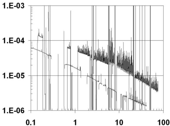
Figure 4: Gas-bremsstrahlung measurements during initial vacuum conditioning of normal (lower curve) and a problematic (upper curve) 5 m long, 8 mm vertical aperture, NEG-coated aluminium ID vessels installed on the ESRF storage ring. Scale units as per figure 3.
