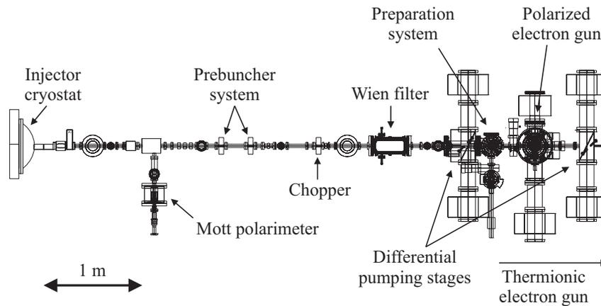
Figure 4: Technical drawing of the planned installation of SPIN at the S-DALINAC. The existing unpolarized thermionic gun is located outside the right edge of the figure; on the far left, the beginning of the cryostat of the superconducting 10-MeV injector linac is shown. The preparation system is placed above the beam line.
