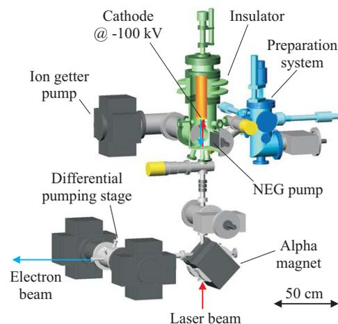
Figure 1: Technical drawing of the core part of the source of polarized electrons. The central UHV chamber contains a highly polished electrode holding the sensitive semiconductor photocathode. The laser beam is incident from the bottom. After a short vertical beam line with a compact quadrupole triplet, the electrons are deflected by an alpha magnet.
