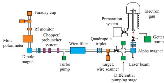
Figure 2: Schematic drawing of the SPIN test setup.
