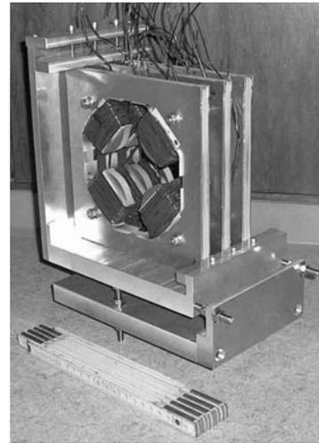
Figure 3: Photograph of a compact triplet of quadrupoles with a total length of only 72 mm and 51 mm aperture.
