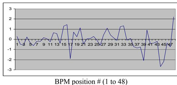
Figure 2. Difference (in microns) between two horizontal orbit measurements, each averaged over 200 samples.
