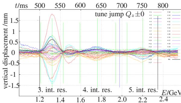
Figure 2: The vertical traces of the beam position monitors are shown (colored for each bpm and in black for RMS) during the energy ramp in the stretcher ring (1.2–2.4 GeV with 4 GeV/s). The correction for the integer resonances causes additional vertical displacements.
