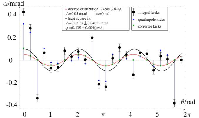
Figure 3: Correction of third integer resonances according to the previous scheme. Each set of samples (green, blue and black dot) represent one dipole segment. The green dots fit smoothly into the desired field distribution (red line). In contrast, the integral kick angles vary strongly from the desired field and a  $\chi^2/\text{dof} = 24.203$  is obtained.
