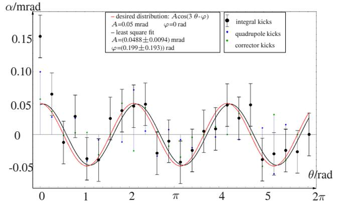
Figure 4: Correction of third integer resonances according to the new scheme. Each set of samples (green, blue and black dot) represent one dipole segment. In comparison with the previous correction, the integral kick angles fit well to the desired field (red line) and a much better  $\chi^2/\text{dof} = 0.925$  is obtained.
