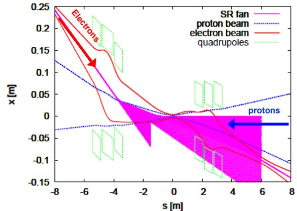
Figure 2: First conservative approach for an IR design with electron triplets. Red: electrons  $20\sigma$  envelope. Blue: protons  $12\sigma$  envelope. Magenta: electron SR fan.
