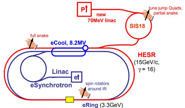
Figure 1: Scheme of the ENC@FAIR (not to scale) for electron-proton collisions.
