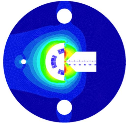
Figure 2: Conceptual cross section design of a superconducting half quadrupole magnet.
