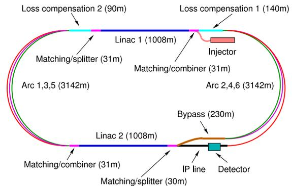
Figure 1: LHeC energy recovery linac configuration.
