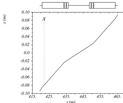
Figure 1: Electron beam orbit in the High Acceptance IR, designed for beam separation. Separation is generated by a crossing angle, dipoles, and offset final quadrupoles.
