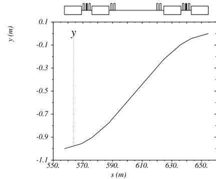
Figure 2: Orbit plot for a DBA dogleg pair in the HA LSS design. The first DBA achromatically bends the beam upwards, while the second reverses this deflection. The scheme displaces the beam vertically without changing angle or vertical dispersion.
