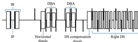
Figure 5: Components of the right side of the LSS. The DS compensation dipole, not used on left side, corrects angle from the weakened DS dipoles.
