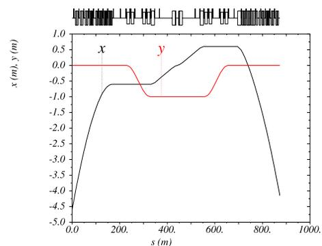
Figure 4: Geometry of the LSS design. For these small angles, the  $s$  axis approximates the  $z$  axis well, and is used to allow MADX to display lattice elements.
