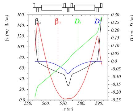
Figure 3:  $\beta$  and dispersion functions in both transverse planes for a single DBA module in the HA LSS design. The cancellation of vertical dispersion, in blue, is clear.
