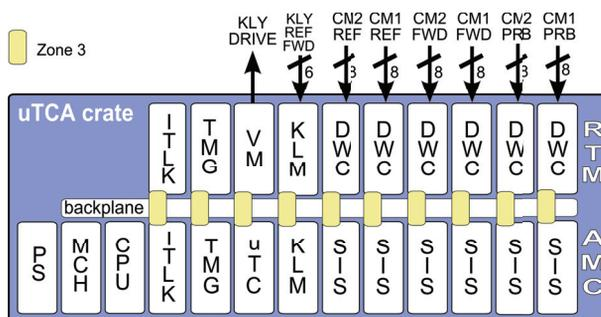
Figure 3: Top view of the MTCA.4 board distribution.
