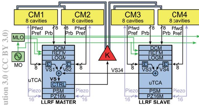
Figure 2: The RF station LLRF master-slave architecture.
