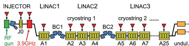
Figure 1: XFEL accelerator overview.
