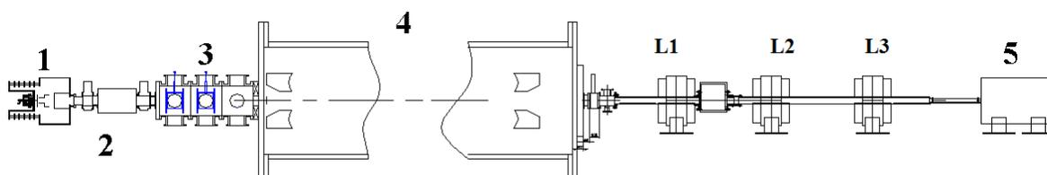
Figure 1: ITEP RFQ HIP-1. 1 - injector, 2 - diagnostic chamber A, 3 - electrostatic lens, 4 - RFQ, 5-diagnostic chamber B, L1,L2, L3 –quadruple lenses.
