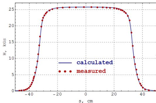
Figure 11: Field longitudinal distribution  $B_y(s)$  at 9.9 kA.
