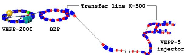
Figure 9: VEPP-2000 accelerator complex after upgrade.
