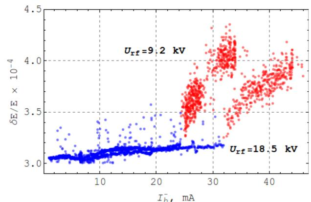
Figure 7: Beam energy spread as a function of beam current @ E=480 MeV.
