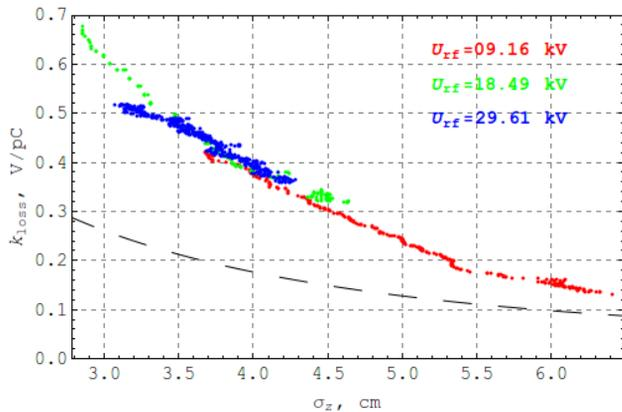
Figure 8: Longitudinal loss factor @ E=480 MeV.
