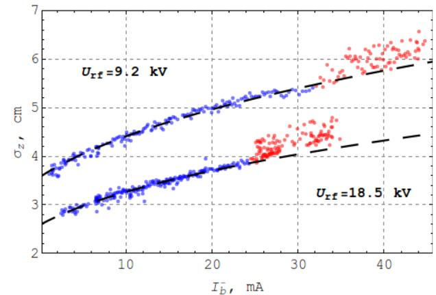
Figure 6: Bunch length as a function of beam current @ E=480 MeV.
