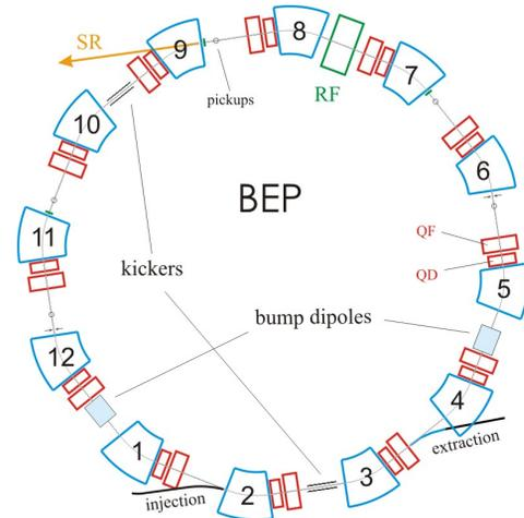
Figure 10: Booster synchrotron BEP layout.
