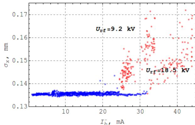
Figure 5: Horizontal beam size on 4MIL CCD (in place with non zero dispersion) as a function of beam current @ E=480 MeV.
