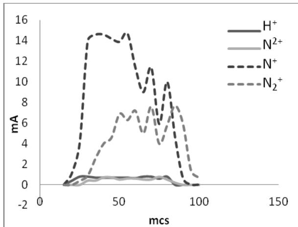
Figure 3: Charge ion distribution in duoplasmatron beam.
