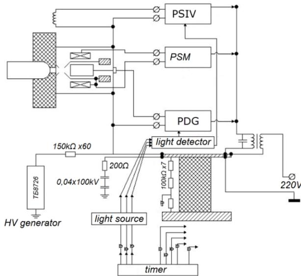
Figure 2: Circuit of duoplasmatron power supply.
