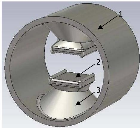
Figure 1. The model of one deflecting cell, where 1 – cavity's shell; 2 – electrode; 3 – electrode's stem.
