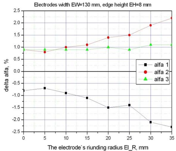
Figure 5. The dependence of deflecting homogeneity on electrode's rounding radius  $El\_R$ .
