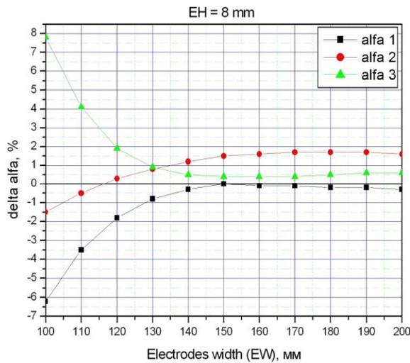
Figure 2. The dependence of deflecting homogeneity on electrodes geometrical sizes. (the angle number corresponds to [5]).
