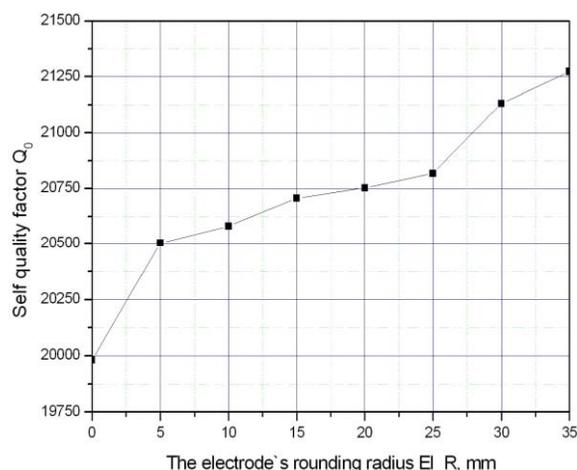
Figure 6. The dependence of self quality factor  $Q_0$  on electrode's rounding radius  $El\_R$ .
