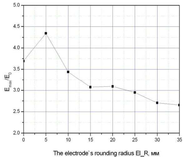
Figure 4. The dependence of  $E_{max} / E_0$  on electrode's rounding radius.
