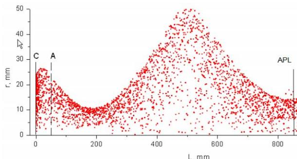
Figure 3: Electron beam propagation;  $I=100$ A,  $U=200$ kV.
