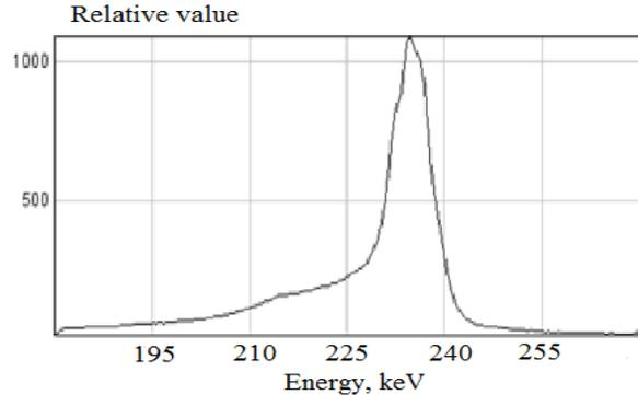
Figure 6: Electron beam energy spectrum for charging voltage 28 kV.
