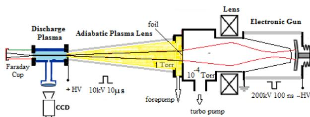
Figure 1: Set up of the adiabatic plasma lens with the ITEP electron gun.
