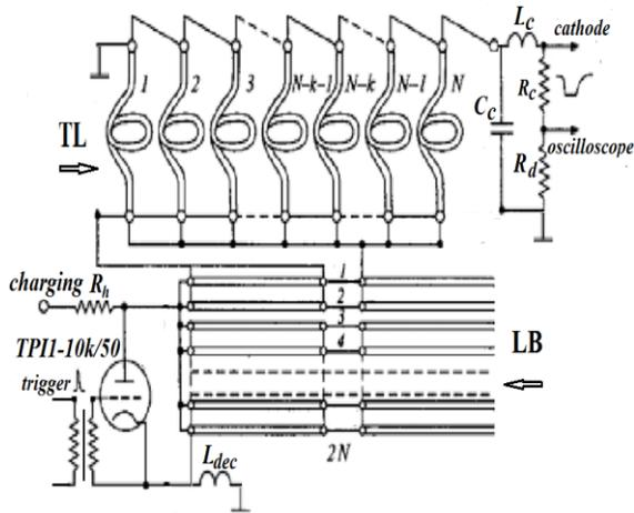
Figure 4: Pulse modulator.
