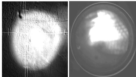
Figure 9: Scintillators luminescence for the lens entrance and exit.
