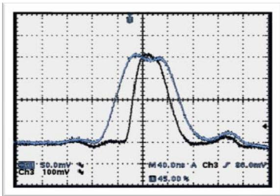
Figure 5: The electron beam current (black curve) and DFL voltage pulse signals.
