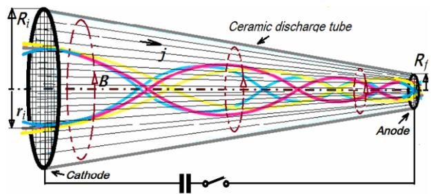
Figure 7: Schematic drawing of the principle and geometry of an adiabatic plasma lens.
