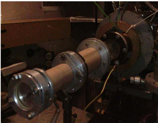
Figure 8: The adiabatic plasma lens (initial part).
