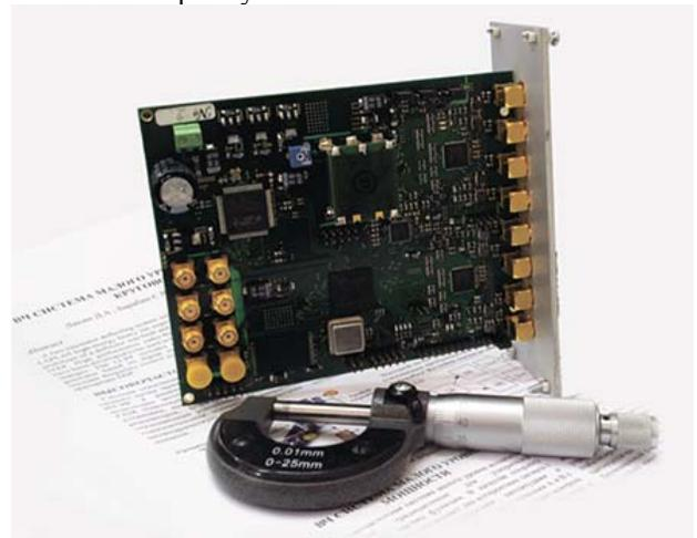
Figure 6: The ADC module.
