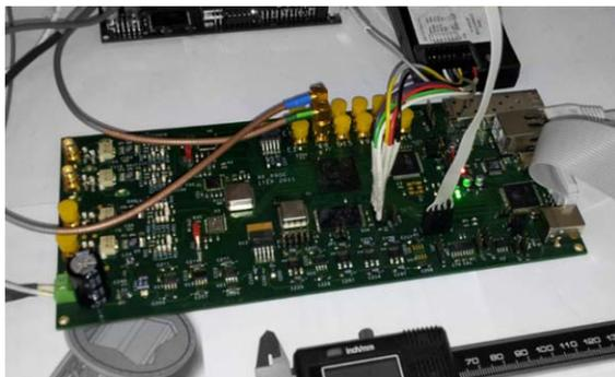
Figure 5: The PCB of the reference generator.
