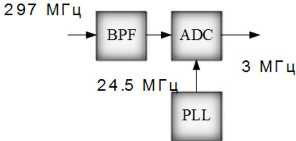
Figure 7: Analog to digital conversion using the IF mode.
