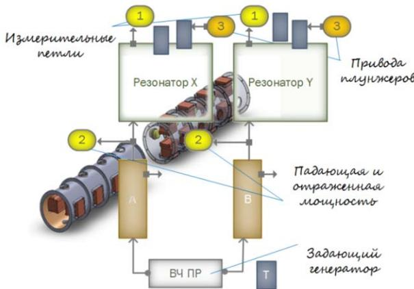
Figure 1: RF system of the beam deflector.
