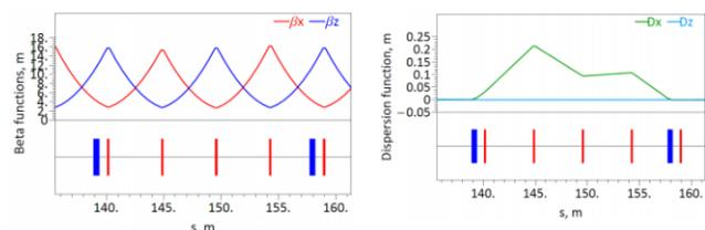
Figure 11: Lattice functions of second horizontal bend in regular part.
