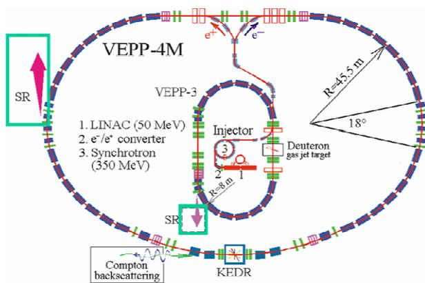
Figure 3: Accelerator Complex VEPP-4M.
