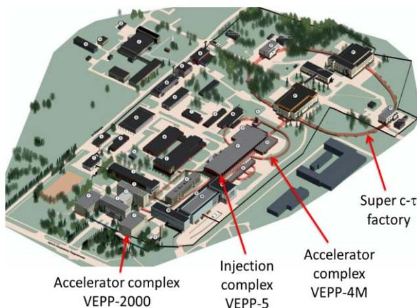
Figure 1: Colliders and Injection Complex in BINP.
