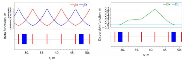
Figure 9: Lattice functions of first horizontal bend in regular part.
