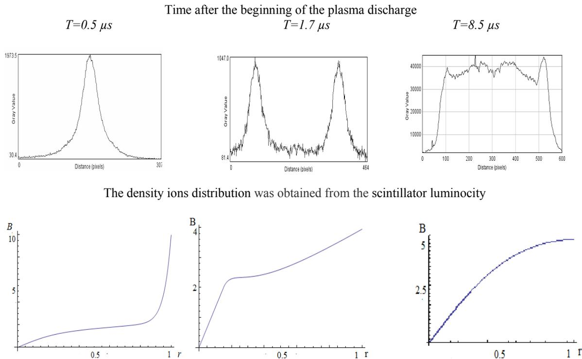
Magnetic field strength obtained by mathematical processing of experimental data
