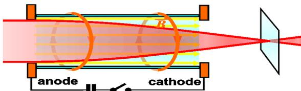
Figure 1: Ion focusing in a plasma lens.
