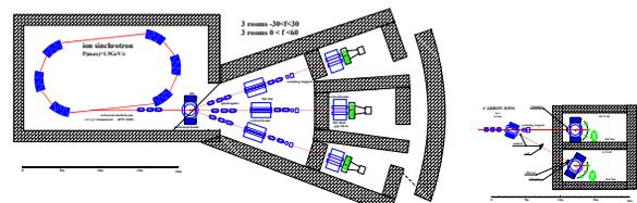
Figure 8. Scheme of transport system for ion therapy center with 6 treatment rooms.
