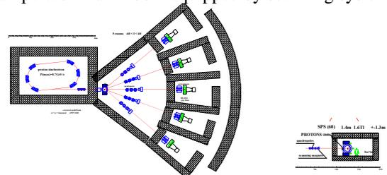
Figure 7. Scheme of transport system for proton therapy center with 5 treatment rooms.
