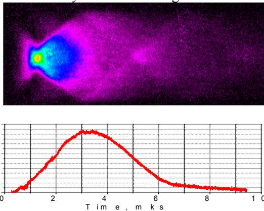
Fig. 1: Time scanning of the discharge luminescence and current.
