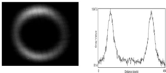
Fig. 5: Light output from scintillator and distribution of ion  $Fe^{+26}$  density at  $1.7 \mu s$  after beginning of discharge at distances of 30 cm for discharge current of 150 kA. The ring diameter is 9 mm .
