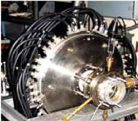
Figure 4: Picture of the plasma lens on the measuring stand.
