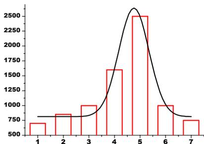
Figure 7: Gauss fit of registered beam profile
