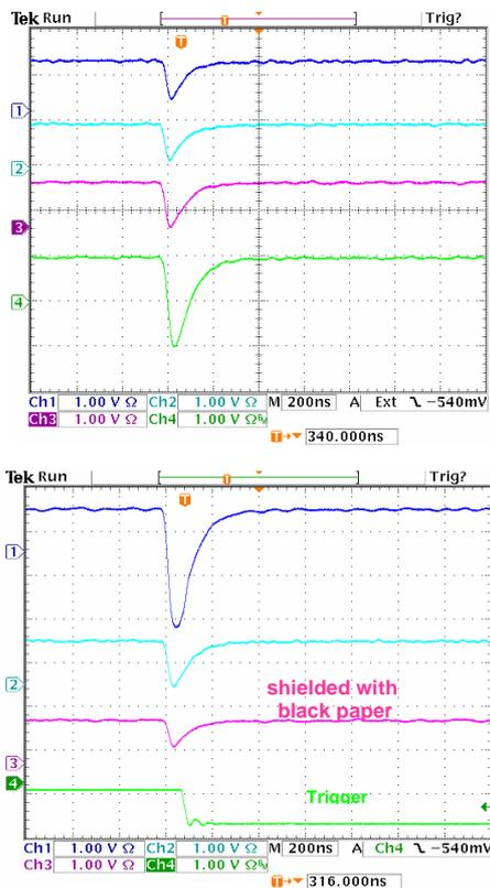
Figure 6: Oscillogrammes of light signals registered at pressure of N<sub>2</sub> of 16 mbar.
