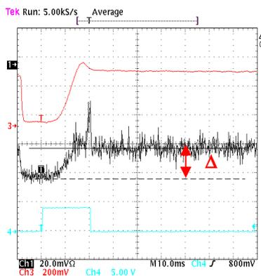
Figure 2: Signals of light intensity measured at COSY ring,  $p = 6 \cdot 10^{-8}$  mbar,  $4.7 \cdot 10^{10}$  p,  $\Delta = 21.2$  mV
