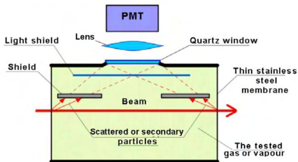
Figure 4: Scheme of gas test chamber
