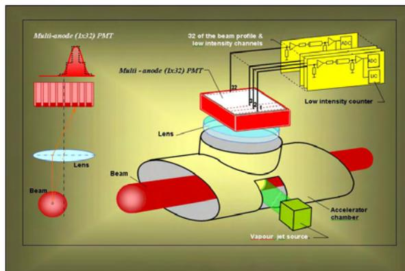
Figure 3: Scheme of beam position and profile monitor
