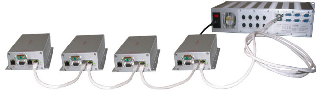
Figure 2: BSC modules connected in a daisy chain and connected to a microIOC-CosyIcon as the central processing unit. To each BSC two Bergoz detectors can be connected (not shown).
