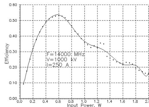
Figure 2: Amplitude characteristic of the klystron.
