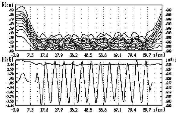
Figure 3: Magnetic field of the klystron and numerical simulations of the electron beam transport.
