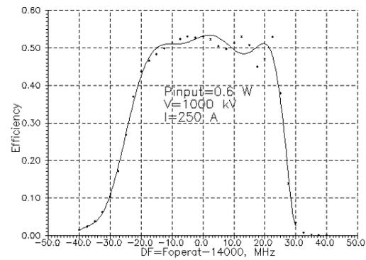
Figure 1: Frequency characteristic of the klystron.
