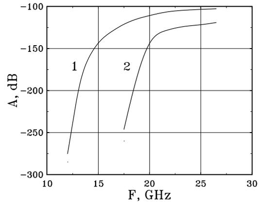
Figure 4: Integral frequency characteristic of the distributed suppression filter composed of ten RF absorbing drift tubes (1 –  $H_{11}$ -mode and 2 –  $E_{01}$ -mode).
