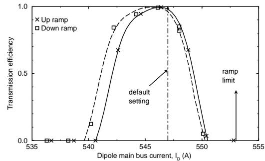
Figure 5: Sextant dipole and quadrupole hysteresis measurement by transmission efficiency scan.
