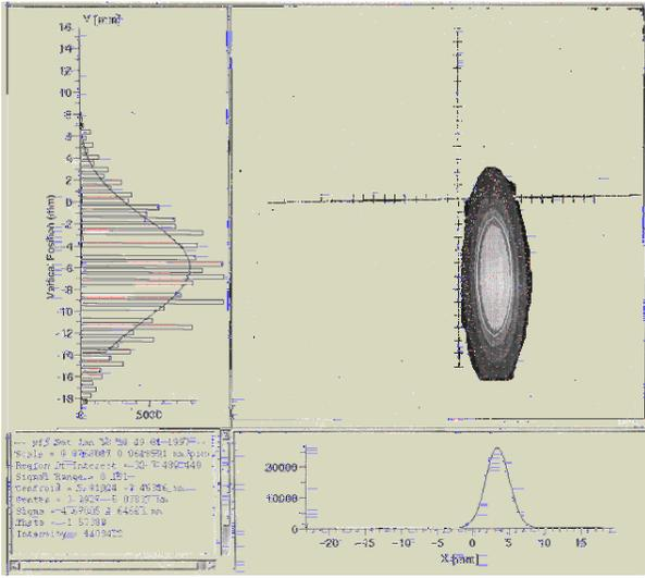
Figure 2: Transverse beam profile in the AtR recorded on flag wf3 (2D image and projections) and IPM (histogram).
