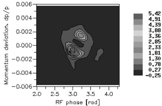
Figure 1: Longitudinal phase space diagram of a Au<sup>77+</sup> beam in the AGS reconstructed with RADON showing imperfect bunch coalescing at an early stage of the test.
