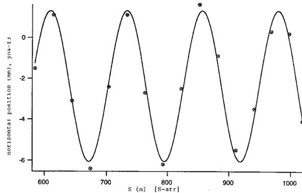
Figure 3: Beam position on the last flag versus perturbation location for Sextant phase advance measurement. The solid line is a sine-wave fit to the data.
