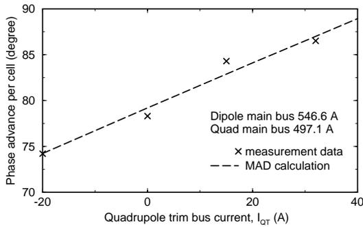
Figure 4: Comparison between the measurement and MAD lattice modeling on horizontal phase advance per cell as a function of arc focusing quadrupole strength.
