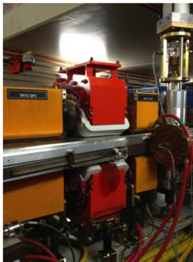
Figure 3: SHD magnet installed between the QF and QD quadrupoles.
