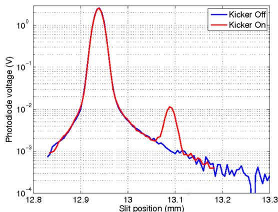
Figure 3: X-ray pulse measurements at a bend magnet beam line 10.3.2 with the kicker on and off. For these measurements, the storage ring was filled with a 350 mA multibunch train and a 4 mA camshaft bunch.
