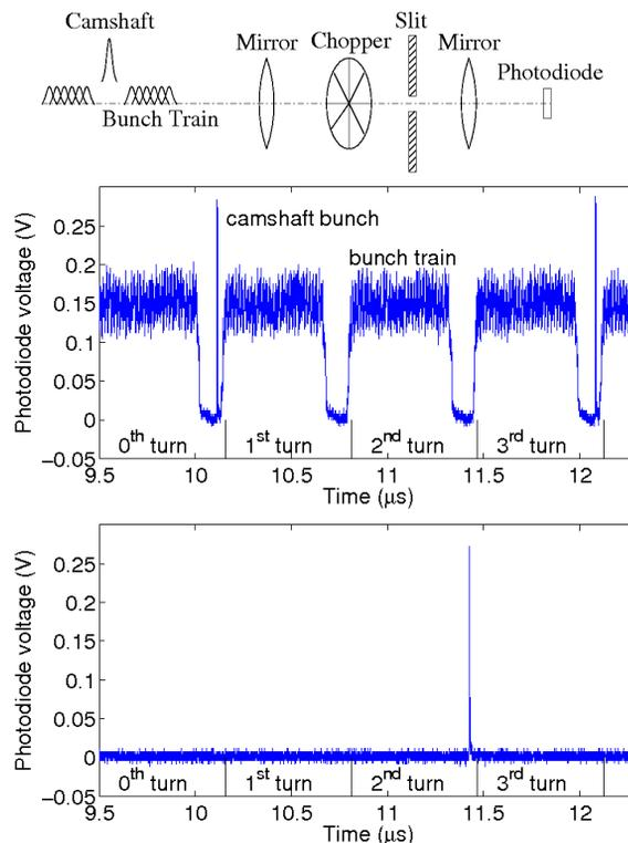
Figure 4: X-ray pulse measurements at an undulator beam line 6.0.1. (Top) Experiment setup; (Middle) On-axis measurement. The 50  $\mu\text{m}$  slit is centered on axis. (Bottom) Off-axis measurement. The slit is off axis by 190  $\mu\text{m}$ .
