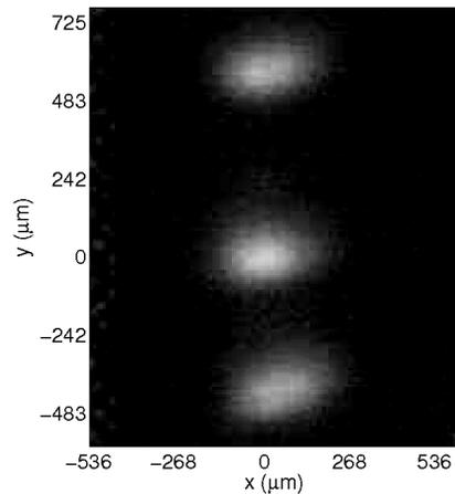
Figure 2: Beam image measurement at synchrotron diagnostic beam line 3.1. For this measurement, the storage ring was filled with a 5 mA single camshaft bunch, and the beam was kicked at the maximum kick-and-cancel frequency.
