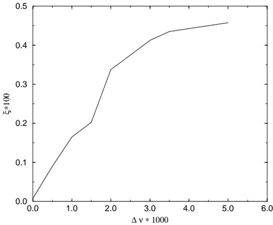
Figure 2: Threshold antiprotons tune shift  $\xi_e$  (vertical axis) due to the electron beam versus the difference of antiproton horizontal and vertical tunes  $\Delta\nu = \nu_x - \nu_y$ .  $B = 10$  kG,  $\nu_s = 0.001$ ,  $N_{\bar{p}} = 6 \cdot 10^{10}$ .
