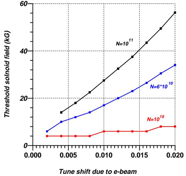
Figure 3: Threshold solenoid field  $B_{thr}$  vs tune shift due to electrons  $|\xi_e|$  at different bunch populations  $N_{\bar{p}} = 1, 6, 10 \cdot 10^{10}$ . Focusing lattice tunes  $\nu_x = 0.585$ ,  $\nu_y = 0.575$ , synchrotron tune  $\nu_s = 0.0012$ , maximum tune spread  $\delta\nu = 0$ , the rms size of  $\bar{p}$  beam  $\sigma_{\bar{p}} = 0.7$  mm.
