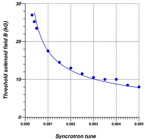
Figure 4: Threshold magnetic field vs synchrotron tune  $\nu_s$ . Solid line is for  $B_{thr} = 12.4[kG]/\sqrt{\nu_s}$ .  $\nu_x = 0.585$ ,  $\nu_y = 0.575$ ,  $\xi_e = -0.01$ ,  $\delta\nu = 0$ ,  $N_{\bar{p}} = 6 \cdot 10^{10}$ ,  $\sigma_{\bar{p}} = 0.7$  mm.
