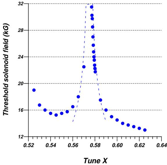
Figure 5: Threshold magnetic field vs horizontal tune  $\nu_x$ . Dashed line corresponds to  $B_{thr} \propto 1/\sqrt{|\nu_x - \nu_y|}$ ;  $\nu_y = 0.575$ ,  $\nu_s = 0.001$ ,  $\xi_e = -0.01$ ,  $\delta\nu = 0.0$ ,  $N_{\bar{p}} = 6 \cdot 10^{10}$ ,  $\sigma_{\bar{p}} = 0.7$  mm.
