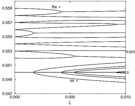
Figure 1: Eigenfrequencies (tunes) of the antiproton bunch oscillation modes versus the antiproton betatron tune shift due to electron beam  $\xi_e$  (horizontal axis). Vertical scale on the left is for fractional part of the tunes  $Re\nu$  (upper series of lines), the right side scale is for imaginary part of the tunes  $Im\nu$  (lower series of lines).
