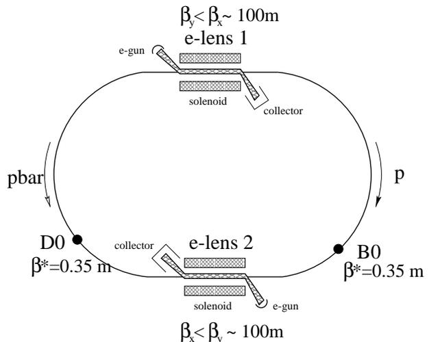
Figure 2: Tevatron layout with two “electron lenses”.
