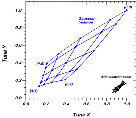
Figure 4: Betatron frequencies (tunes) in the  $\bar{p}$  bunch for particles with different betatron amplitudes  $(X, Y)$ . The head-on collision case (large leaf) and the case with compensation by the electron beam (small leaf, displaced for clarity) [2] are shown. Tune shift is in units of  $\xi^p$ , betatron amplitude is in units of the bunch transverse size  $\sigma$ .
