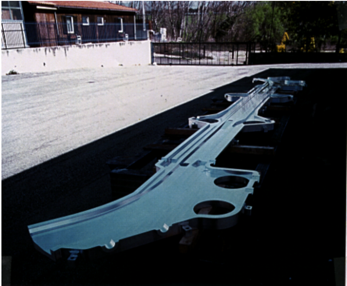
Figure 3: Arc Al vacuum vessel, one half, before welding at CECOM.
