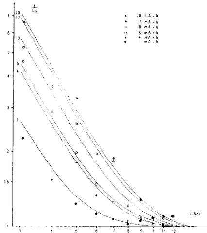
Fig. 3. Ratio between experimental and theoretical bunch length as function of energy and current per bunch.
