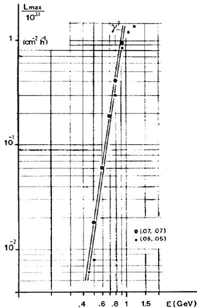
Fig. 5. Maximum luminosity as function of energy.
