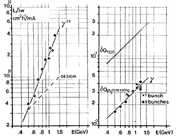
Fig. 6.  $L/i_w$ ,  $\delta Q_{R, V}$  per crossing and  $Q_{TOT}$  as functions of energy.
