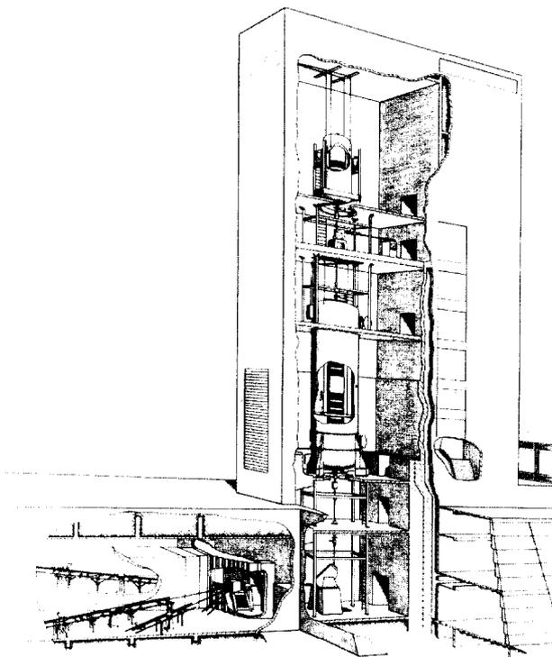
Fig. 10. Three stage 22MeV Pelletron accelerator facility built by NEC for the University of Sao Paulo, Brazil.
