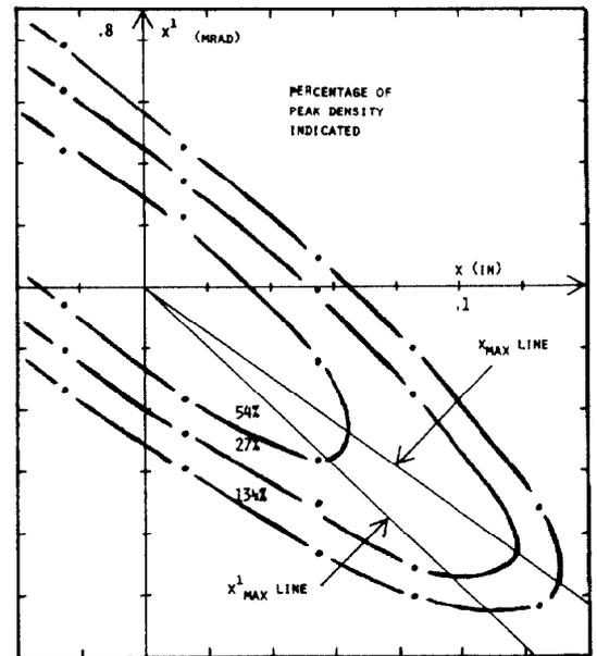
Fig. 6. Phase Plane Equi-Density Contours.
