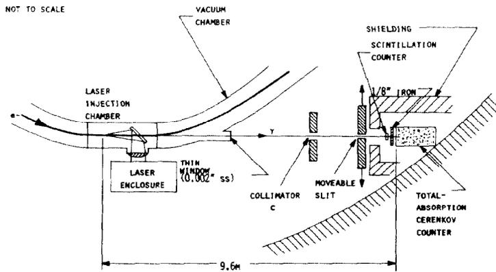
Fig. 1 (left). Schematic Diagram of Experimental Setup.
