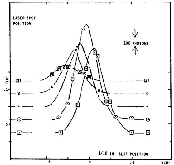
Fig. 5. Horizontal Slit Scans at Various Fixed Laser Positions.
