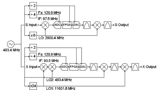
Figure 1: Frequency generation scheme for IF, LO and Fs.
