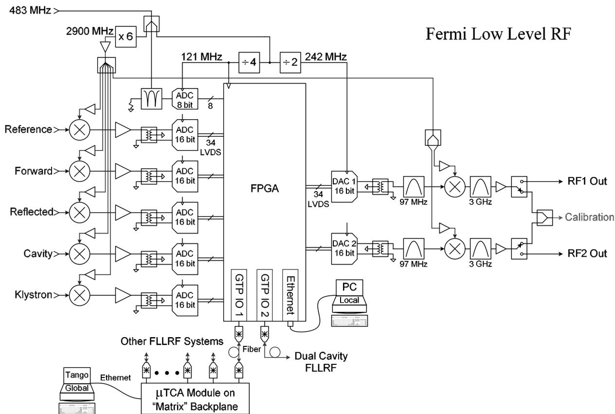
Figure 3: Fermi LLRF control system architecture for S-band section.
