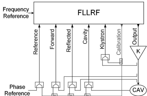
Figure 2: Fermi LLRF control system configuration.
