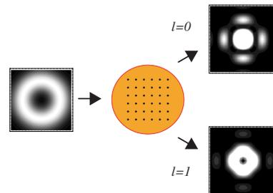
Figure 3: The far field patterns of a pepperpot can be used to distinguish different phase topologies of similar intensity patterns.
