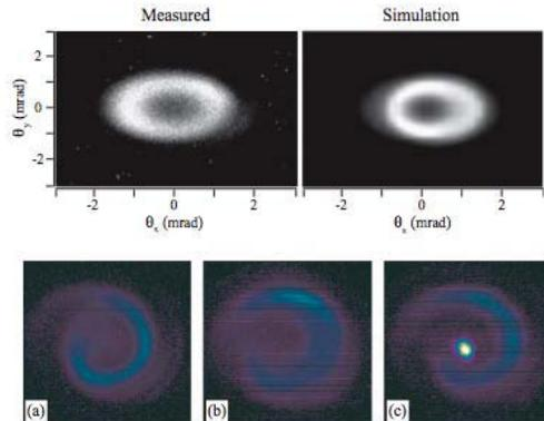
Figure 1: Spiral intensity profiles from VISA. A HeNe alignment laser identifies the e-beam axis in the right, lower image.
