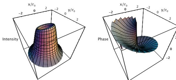
Figure 6: Transverse field at undulator exit for helical density perturbation.
