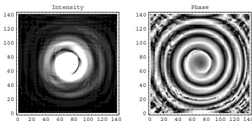
Figure 5: The complex field from VISA SASE at a single longitudinal slice from a Genesis 1.3 simulation with a helically perturbed e-beam.
