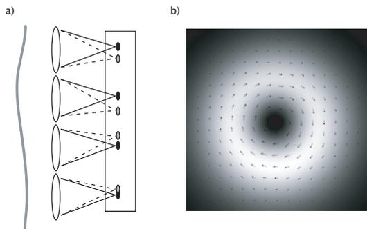
Figure 4: a) A basic microlens array. The focal points of an incoming signal wave with a curved phase front are compared with those of a reference wave. The shift in the focal point is related to the phase curvature over each lens. b) An example  $l=1$  mode (courtesy A. Mancuso).
