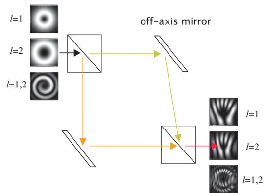
Figure 2: Schematic representation of a simple skew interference measurement used to reveal the azimuthal mode content OAM modes. Each input beam (left) interferes with itself and produces the signature fringe patterns (right).
