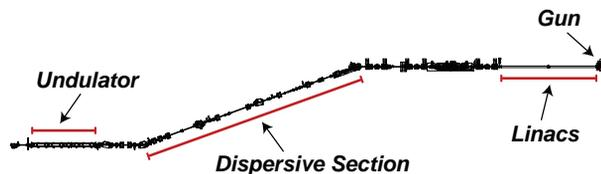
Figure 1: A schematic of the VISA beamline.
