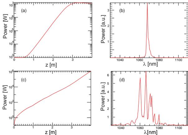
Figure 4: Gain curve and spectrum for seeding (a,b) and SASE (c,d) for comparison, for the same electron beam.
