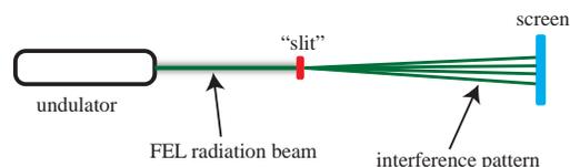
Figure 3: A schematic of the transverse coherence measurement.
