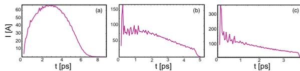
Figure 2: Current profiles at the undulator entrance for three different stages of compression, from simulation.
