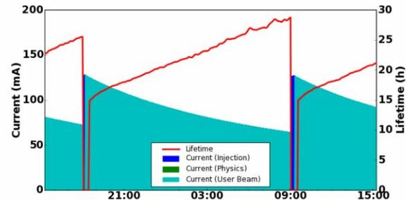
Figure 1: 24 hours of operation; refills at 6pm and 9am.
