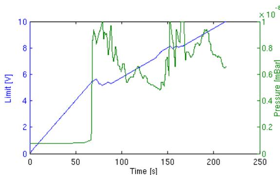
Figure 2: First booster RF ramp following a shutdown. Power limit control (left, blue) and pressure (right, green)
