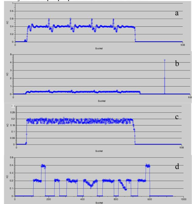
Figure 3: Storage ring fills: a) two-thirds fill, b) hybrid fill, c) smoothed two-thirds fill, d) “diamond” fill
