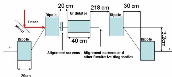
Figure 4. Laser heater layout
