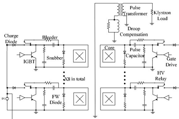
Figure 5. Schematic of solid state modulator.
