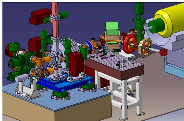
Figure 3: Photoinjector Layout. Valves are represented in green, pumps in red and some supports are hidden.
