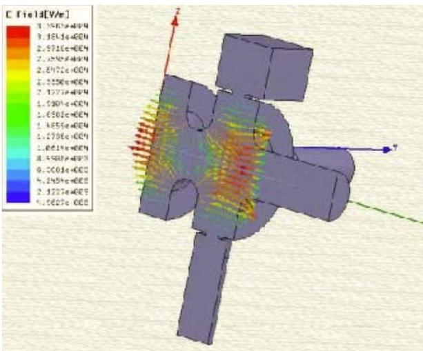
Figure 2. Fields in HFSS simulation of FERMI RF gun.
