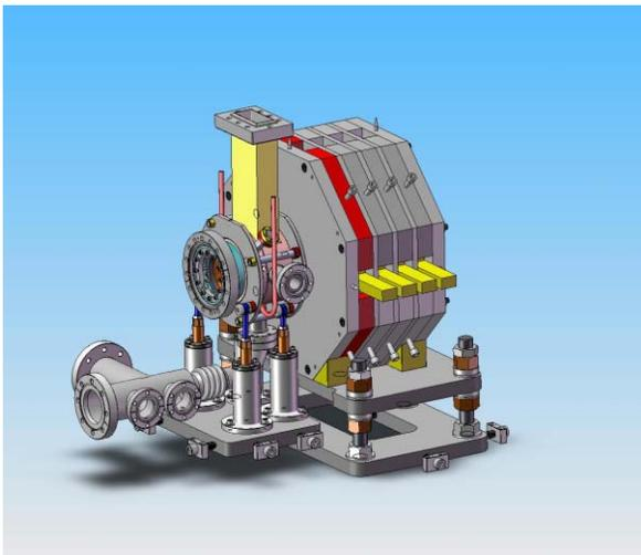
Figure 1. FERMI photoinjector: gun, solenoid, supports.
