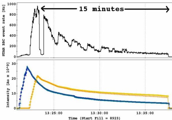
Figure 3: A 15-minute Au-Au store at  $\sqrt{s} = 9.18$  GeV/u, showing blue and yellow beam intensities and STAR BBC counter collision rates. Beams were uncogged and recogged at the start of the store; vernier scans in both planes were performed during the store.
