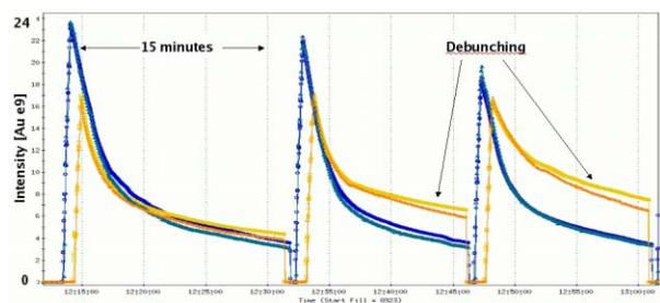
Figure 2: Au beam lifetime at  $\sqrt{s} = 9.18$  GeV/u (blue and yellow rings), with a slow exponential decay component of 20 minutes and a fast exponential decay component of 2 minutes. Bunched and total beam currents are displayed; debunching is clearly visible, so momentum aperture is larger than the RF bucket size.
