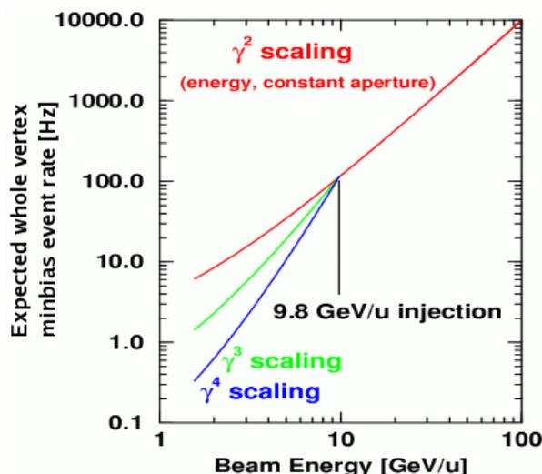
Figure 1: Scaling of RHIC minbias event rate (or luminosity) into the low energy regime. Energies of interest are  $\sqrt{s} = 5\text{--}50$  GeV/u, or beam kinetic energies of 1.6–24.1 GeV/u. Determination of low energy collision rate scaling with  $\gamma$  is important for RHIC low-energy run planning.
