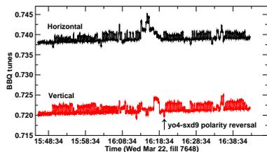
Figure 4: Yellow BBQ tunometer data acquired for scans of yellow ring bumps in arcs 10/11, 12/1, 2/3, 4/5, 6/7, and 8/9 o'clock. The bump at 16:19 indicates a polarity reversal of chromaticity sextupole yo4-sxd9.
