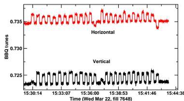
Figure 3: A zoom of the blue BBQ tunometer data acquired for scans of blue ring bumps in arcs 6/7, and 8/9 o'clock, showing detailed bump configurations for correctly wired chromaticity sextupoles.
