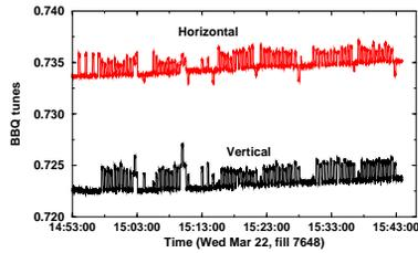
Figure 2: Blue BBQ tunometer data acquired for scans of blue ring bumps in arcs 10/11, 12/1, 2/3, 4/5, 6/7, and 8/9 o'clock. Anomalies at 15:02 and 15:09 are the result of bumps not being removed, and are not due to mis-wired sextupoles.
