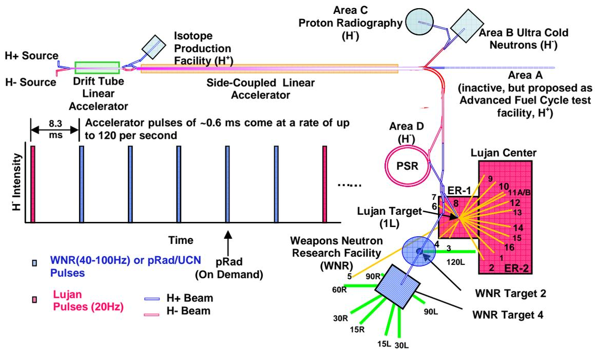
Figure 1: Schematic representation of the LANSCE User Facility at TA-53
