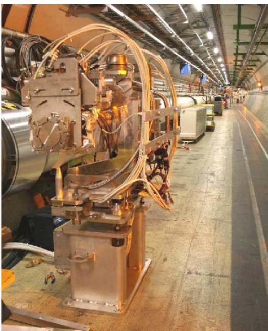
Figure 4: Photograph of LHC collimator installed on its base-support assembly (base-support and quick plug-in).
