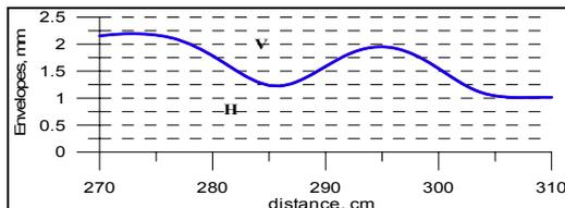
Figure 8:  $^{12}\text{C}^{6+}$  beam envelopes near inflector.
