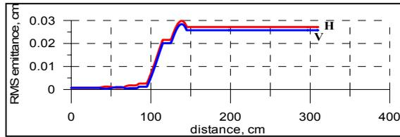
Figure 6. Horizontal (H) and vertical (V)  $^{12}\text{C}^{6+}$  beam emittances in the rotational frame. Non-tilted lenses.
