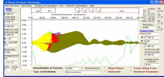
Figure 4: Results of macro particle simulation for  $^{12}\text{C}^{6+}$ . Green line shows distribution of magnetic field.
