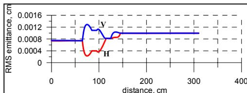
Figure 7: Horizontal (H) and vertical (V)  $^{12}\text{C}^{6+}$  beam emittances in the rotational frame. Tilted lenses.
