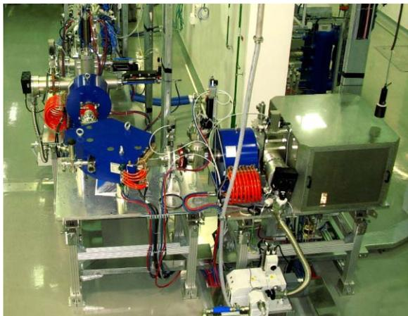
Figure 1: ECR Ion Source with LEBT installed at SARAF
