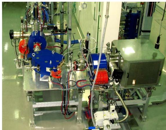
Figure 2: ECR Ion Source (covered by RF cage) with LEBT at SOREQ
