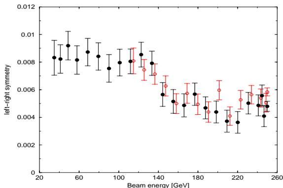
Figure 3: Both data sets in the plot are the polarization measurement as a function of beam energy from two consecutive ramps. Both show a step of left-right asymmetry reduction around 136 GeV where the first strong intrinsic spin resonance beyond 100 GeV at  $G\gamma \sim 260.7$ .
