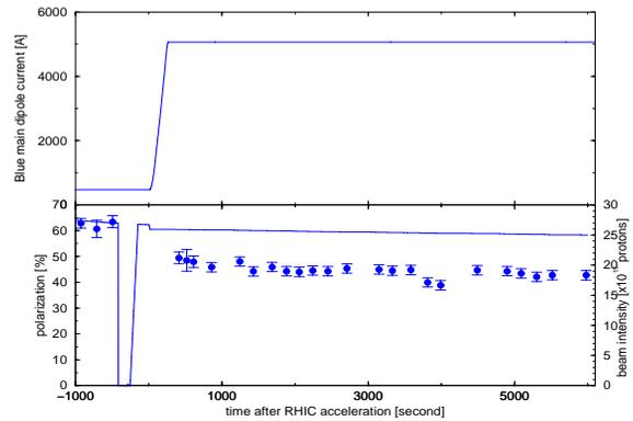
Figure 2: The top plot shows the beam energy in unit of  $G\gamma$  as a function of the time from the beginning of the RHIC acceleration. The bottom plot shows the beam current and polarization measured in the Blue ring. The beam polarization at injection is around 65% and beam polarization at store is about 46%.
