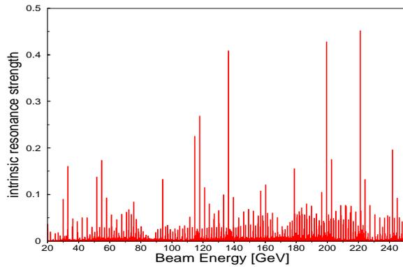
Figure 1: RHIC intrinsic spin resonance strength as a function of beam energy. This is calculated with a  $2\text{ m } \beta^*$  at STAR and PHENIX,  $3\text{ m } \beta^*$  at Brahms,  $10\text{ m } \beta^*$  at PHOBOS and  $5\text{ m } \beta^*$  at the RHIC absolute polarimeter [10].
