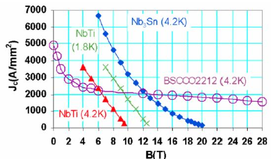
Figure 1: Critical current as a function of field for NbTi, Nb<sub>3</sub>Sn and Bi-2212 conductors.
