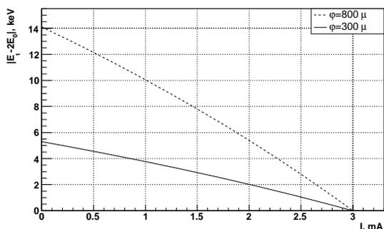
Figure 2: Interaction energy shift versus beam current. Impact parameter is zero at beam current 3 mA.
